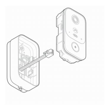
9. Gently insert the main assembly into the wall mount assembly, ensuring that wires are not pinched and there is no excess cable in the doorbell. Firmly press the main assembly until it is completely seated.
