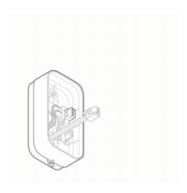
8. Connect the Ethernet cable to the Ethernet port on the back of the main assembly.
