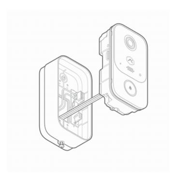
10. Fasten the security screw at the bottom of the wall mount assembly.
