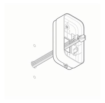
7. If installing chime wires, insert the chime wires into terminals and use a screwdriver to secure them.
